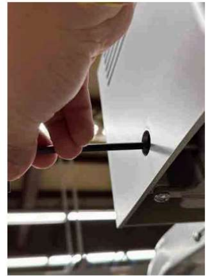
24.10 Left screw: To adjust rotation
